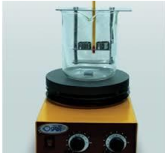
Fig.6 Ring and ball apparatus for softening point
