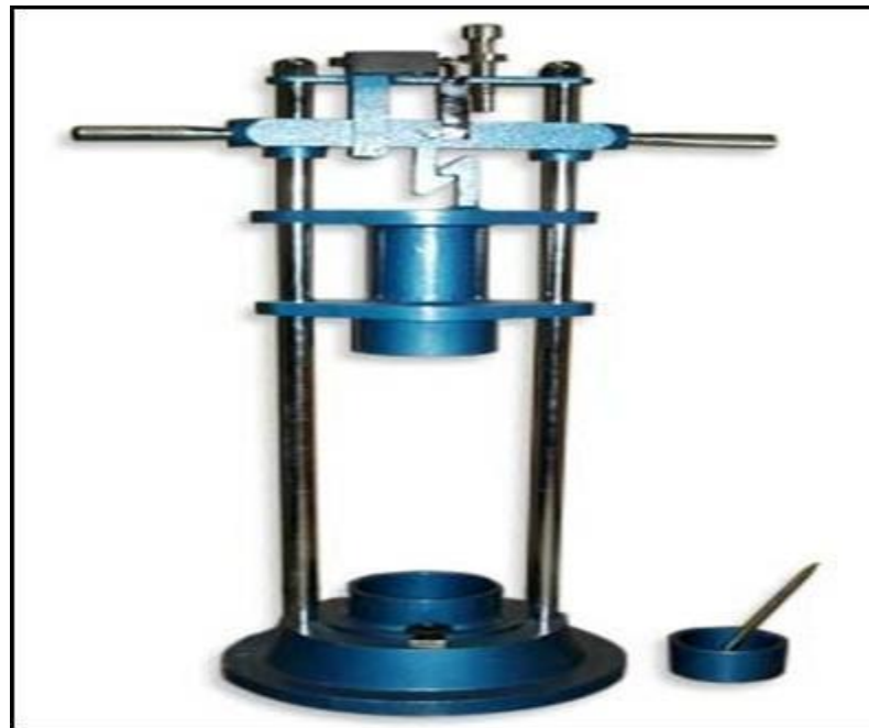
Fig.2 Aggregate impact test apparatus
