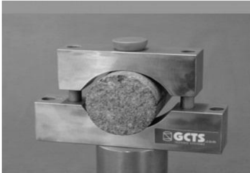
Fig.2 Indirect tensile strength of rock specimen (Brazilian test)
