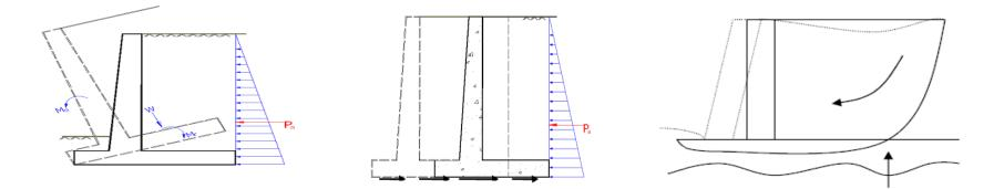
**Typical Failure Modes of Retaining Wall**
