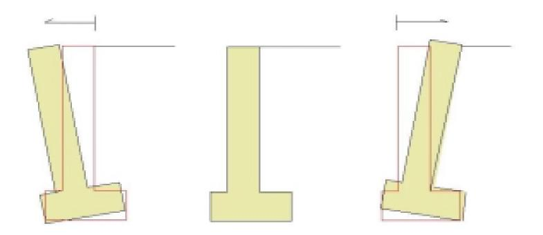
Active Case (Wall moves away from soil) At Rest Case (No movement) Passive Case (Wall moves into soil)
