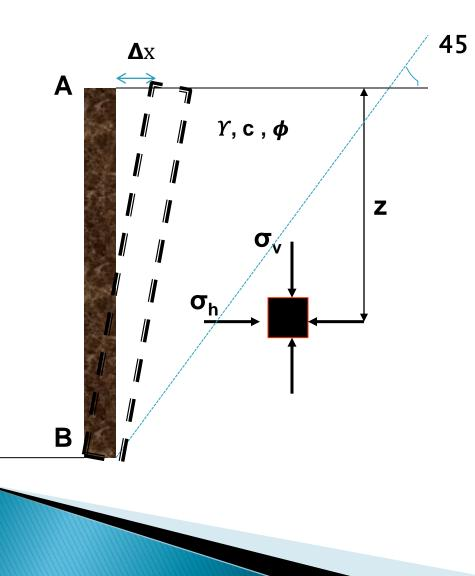
If the wall is pushed into the soil mass, the principal stress  $\sigma_h$  will increase. On the verge of failure the stress condition on the soil element can be expressed by Mohr's circle b.
