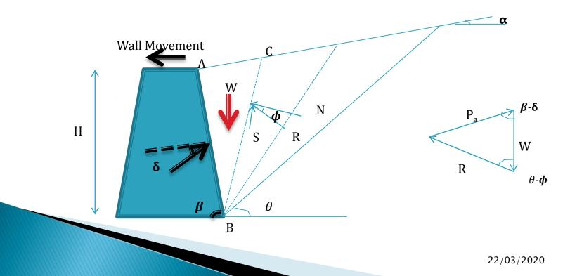
$$K_{a} = \frac{\operatorname{Sin}^{2} (\beta + \phi)}{\operatorname{Sin}^{2} \beta . \operatorname{Sin} (\beta - \delta) \left[ 1 + \sqrt{\frac{\sin(\phi + \delta) . \sin(\phi - \alpha)}{\sin(\beta - \delta) . \sin(\alpha + \beta)}} \right]^{2}}$$
