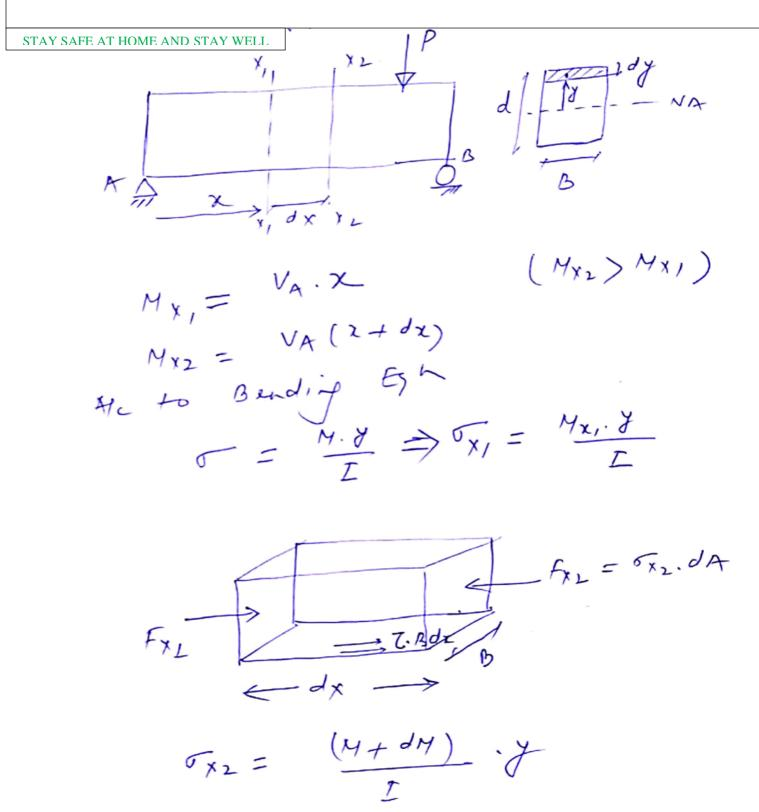
FXI + T.B.dx = Fx2 T.B.dx = / (M+JM). & -M.8 JAA T.B.dx = dm . J. dA  $T = \frac{V}{IB} \cdot y dA$  $\int Z = \frac{V}{I^{\prime}R} \cdot A \cdot y \int$ shear fire at the Section Where shear story measured Homent & meeting & X-seefor about N.A WINTE B X-section at that point where shear Stron measured Area & the point (Above or below) when shear Stown measured Distance & Centrold & abone area from the Neutral ax 15
